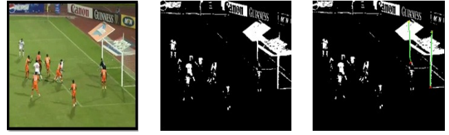
Figure 2. Hough transform detection for the vertical goal posts
